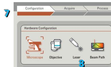
***If you are using the Argon laser, do NOT forget to put the digital power slider at 20% (50% for FRAP experiments).***
